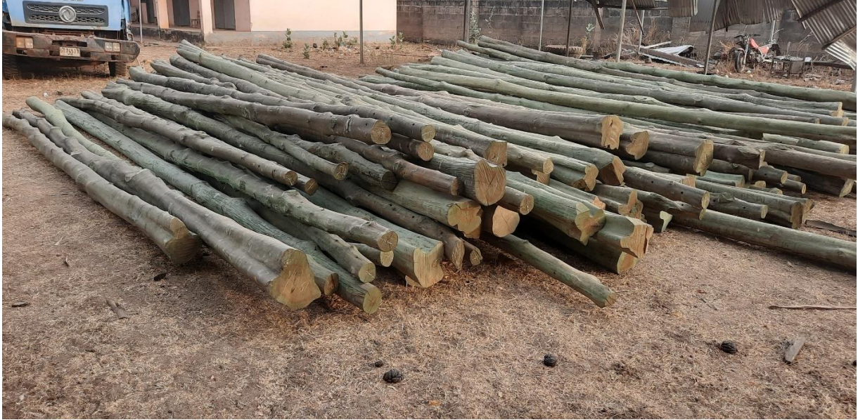
153NO. WOODEN LOW TENSION POLES PROCURED AND DISTRIBUTED UNDER (DACF-RFG)
